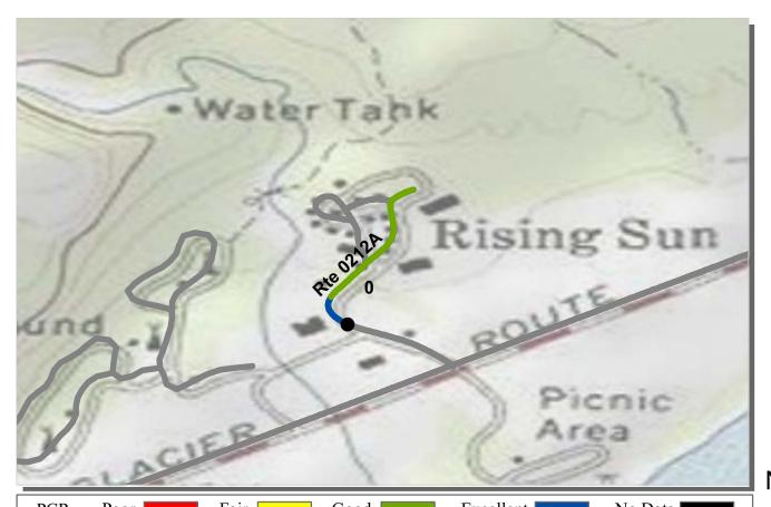
Excellent | No Data **PCR** Fair [ Good | Poor (0 - 60)(61 - 84)(85 - 94)(95 - 100)\* If the PCR rating is not available for a section, the SCR rating will be displayed. See appendix for definitions and formulas.
