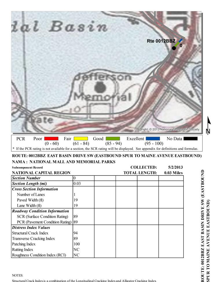
Structural Crack Index is a combination of the Longitudinal Cracking Index and Alligator Cracking Index.
