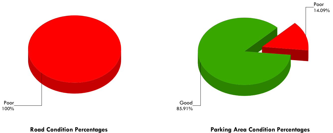
Figure 1: Pavement Condition Rating Breakdown for Paved Roads and Parking Areas
