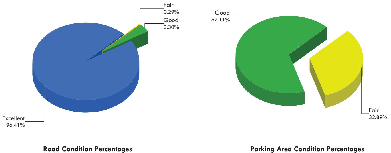
Figure 1: Pavement Condition Rating Breakdown for Paved Roads and Parking Areas
